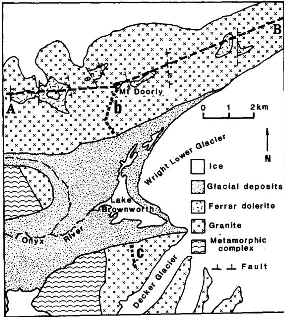
Fig. 4. Geological sketch map of the lower Wright Valley and part of the Mt. Doorly spur. Modified after McKelvey and Webb [22]. The vertical sampling profile up Mt. Doorly (*b*) and that up Mt. Newall (*c*) which lies just off the map to the south, are indicated, as well as the projection line of the cross-section *A-B* which is shown in Fig. 5.
