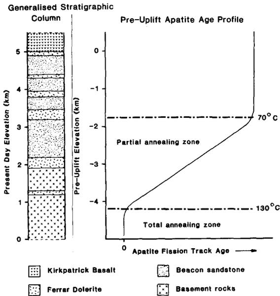
Fig. 7. Generalised stratigraphic column for south Victoria Land [27–31] and reconstructed pre-uplift apatite age profile at Mt. Doorly. The “break in slope” which represents the base of the partial annealing zone then lay at a depth of 4–4.5 km. It now lies at an elevation of about 800 m, inferring an uplift of 4.8–5.3 km.
