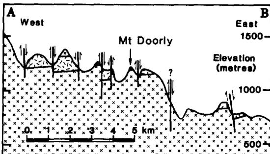
Fig. 5. Geological cross-section through the Mt. Doorly spur showing the offset dolerite sills due to normal step-faulting across the mountain front. The projection line of the cross-section *A-B* is marked in Fig. 4. The question mark indicates that the exact position, not the existence of the fault is in doubt.
